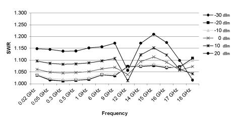
Figure 2. Typical SWR for the E9322A and E9326A sensors at various power levels.
