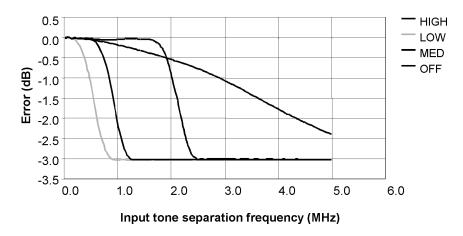
Figure 7. E9322A and E9326A error in peak-to-average measurements for a two-tone input (high, medium, low and off filters).
