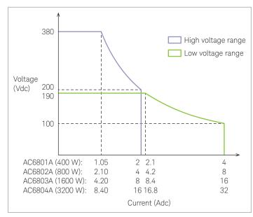
AC6800 steady-state AC output characteristic
