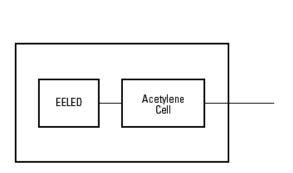
Figure 1. Wavelength calibrator block diagram
