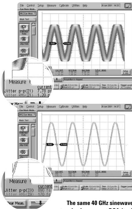
The same 40 GHz sine wave captured using current DCA (top) and now with 86107A precision timebase module (bottom).
