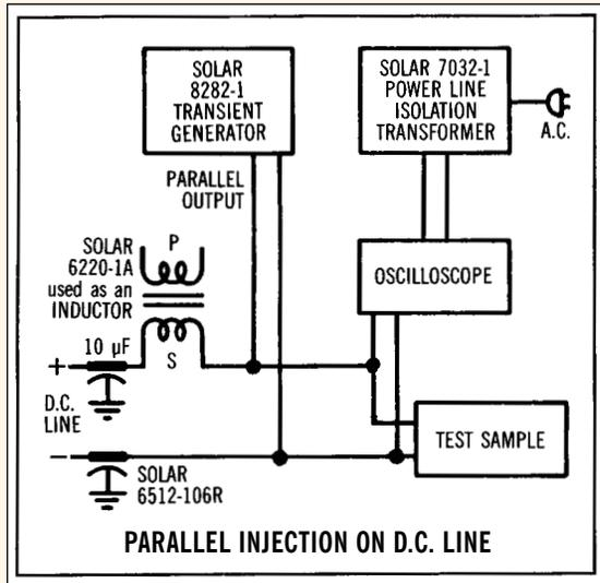
**Adjustable Peak Amplitude:** Up to 600 volts for 0.15  $\mu$ S, 5.0  $\mu$ S and 10.0  $\mu$ S durations into five ohm non-inductive load.
