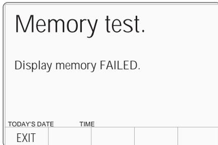
If a failure is reported, rectification will require access to the internal circuitry, so no further user action is recommended, except to report the result to your Wavetek Service Center.
