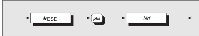
**\*ESE** enables the standard defined event bits which will generate a summary message in the status byte. Refer to Section 6; Subsection 6.5.
