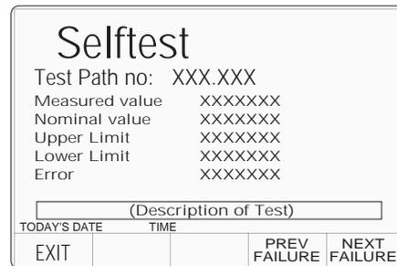
**N.B.** If the cause of failure is not immediately obvious, and it is intended to consult your Wavetek Service Center, please ensure that you *either*: copy the details from the screen for all the reported failures, *or*: print out the results.
