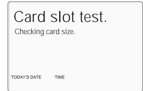
Once the size check is completed, the 9500 starts on a 'read/write' check; meanwhile the display changes to:
