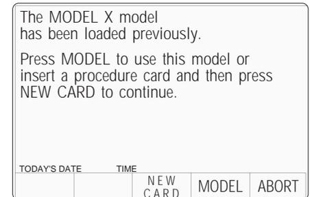
A choice is given: whether to use the loaded procedures, or to insert a new card to load a different model's procedures.
