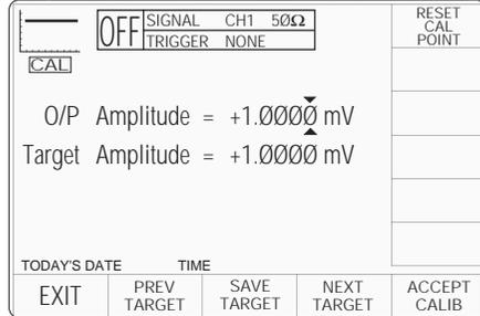
This screen initially shows the value to which the 9500 output is presently set, and the value of the selected target amplitude (whether 'default' or 'saved'). Note that on these values, triangular cursors indicate which digit will change when using the cursor keys or spinwheel. When transferring, using the 'tab' key, the cursor always moves to the least significant digit on the other value.
