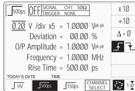
The above default screen has auto-selected the frequency of 1MHz with a rise time of 500ps. Frequency is variable between 10Hz and 2MHz. Deviation has defaulted to zero, and output voltage to 1.0000Vp-p.
