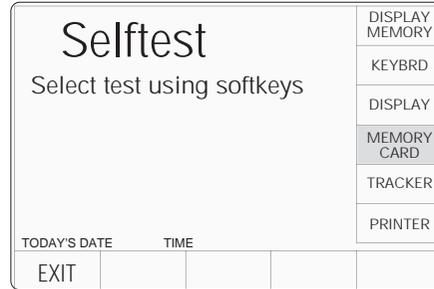
Pressing the MEMORY CARD key on the 'Select test' menu screen transfers to the 'Card slot test.' screen. This invites a user to select the memory card slot to be tested, and presents an 'Overwrite' warning:
