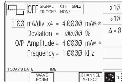
The above default screen has auto-selected the symmetrical square waveform, as indicated by the icon in the top left corner. Frequency is variable between 10.000Hz and 100.00kHz. Frequency has defaulted to 1kHz, deviation 'Δ' to zero, and output current to 4.0000mA<sup>p-p</sup>. The Duty Cycle is fixed at a nominal 50%.
