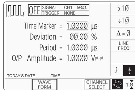
The above default screen has auto-selected the square waveform, as indicated by the icon in the top left corner. Square waveform Period is variable between 10ns and 50s (sine waveform is used above approx 100MHz). Sine waveform Period is variable between 500ps and 10ns (variant 9500/1100 — for other variants refer to specifications in Section 7). Period has defaulted to 1μs (square), deviation 'Δ' to zero, and output voltage to 1.0000Vp-p. The Duty Cycle is fixed at a nominal 50%.
