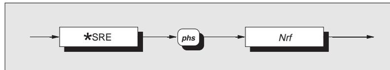
\*SRE enables the standard and user-defined summary bits in the service request byte, which will generate a service request. Refer to Section 6, Subsection 6.5.
