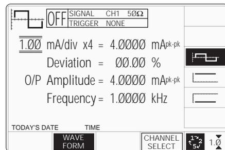
Both polarities of DC Current output are listed merely as different waveforms. As an example, pressing the
