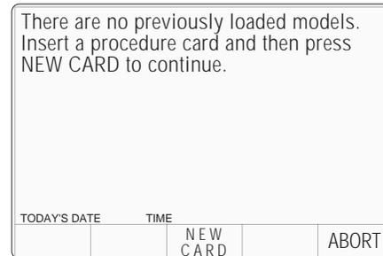
In this case, insert the card required for the UUT into the 'Procedure' slot, push gently home, and press the 'NEW CARD' screen key for the sequence to continue.
