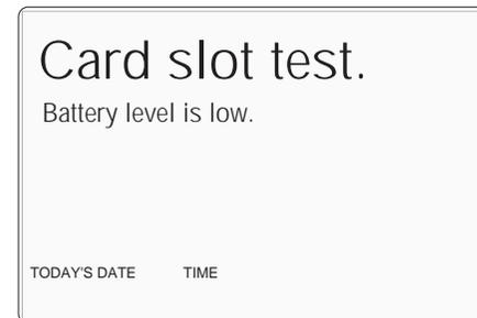
If there is no battery in the card, or if the battery cannot support read/write operations, then the statement will be 'Battery level is dead.'
