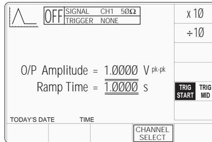
The 9500 has auto-selected a Ramp Time of 1.0000s. Trigger is auto-selected: 'TRIG START', not 'TRIG MID'. O/P Amplitude is fixed at 1.0000V.
