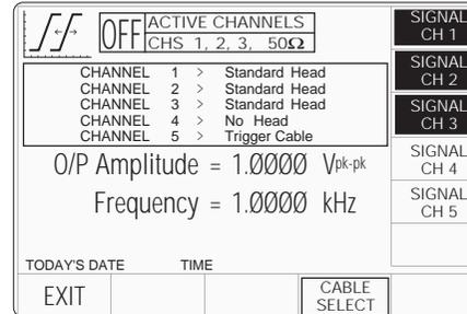
Neither channel 4 nor 5 has an active head fitted. The highlights on channels 1, 2 and 3 indicate that only these channels have heads active (confirmed by the legend in the top central box), and for these zero skew can be used. Toggling any one of these soft keys deselects and reselects that channel. Note that the function cannot operate with only one channel selected, which will cause an error message to appear on the screen.
