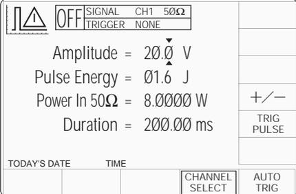
The above default screen has auto-selected the positive pulse waveform, as indicated by the icon in the top left corner. Amplitude is variable between 5 Volts and 20 Volts (default). Pulse Energy is variable between 1.6 Joules (default) and 50 Joules. Power into 50Ω and Pulse Duration are calculated from the voltage and energy settings.
