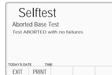
If there were no failures up to the point of aborting, this is shown on the screen.
