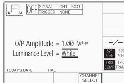
The above default screen has auto-selected 625 lines / 50Hz and triggers will be from composite video. Amplitude has defaulted to a luminance level of 'White' at 1.0V p-p.
