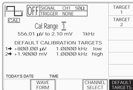
When you select target 2 by pressing its soft key, the Target Amplitude and Frequency will be displayed below the current Output Amplitude as shown in the following **Adjustment** screen illustration:
