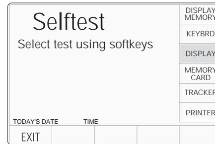
Selecting 'DISPLAY' transfers to the 'Display test.' screen. This invites a user to use the front panel 'tab' (⇨) key to move the dark band down the screen, up to the top, and down again, thus testing all the display elements on the screen:
