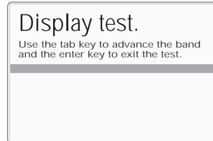
The screen text will shift automatically so as not to obscure the band as it jumps back to the top of the screen. If there are elements of the screen which do not show light in the light background or dark in the dark band as it is advanced down the screen, then this implies a failure. Rectification will require access to the internal circuitry, so no further user action is recommended, except to report the result to your Wavetek Service Center.
