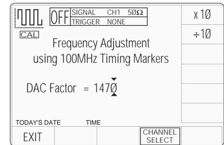
1. **9500** In the **Special Cal** screen, press the **Adjust FREQ** soft key on the bottom row. This transfers to the **Frequency Adjustment** screen:
