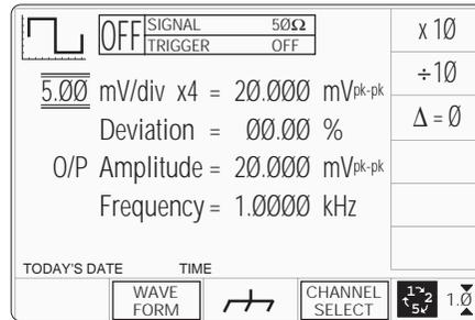
**Fig. 4.3.4.1 Manual Mode Power-Up Screen for Single-Channel Variant**
