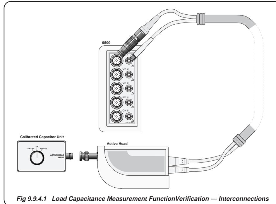
**Fig 9.9.4.1 Load Capacitance Measurement Function Verification — Interconnections**
