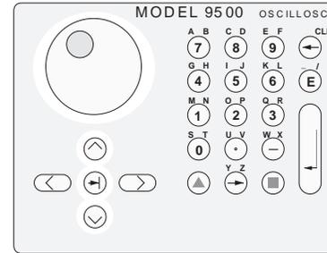
Fig. 4.4.13 Barred Cursor Control Keys
