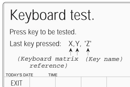
The 'Keyboard matrix reference' (X,Y) relates to the electronic matrix which is used to transfer keypress information to the internal processor, and does not relate closely to the physical layout of keys. The 'Key name' (Z) is the name, in words, which describes the last key to be pressed.
