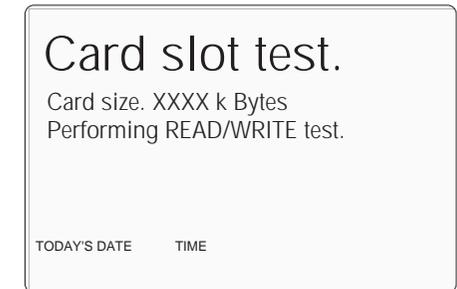
After the read/write check, the 9500 starts on a 'walking ones' check, and the message on the display changes to:
