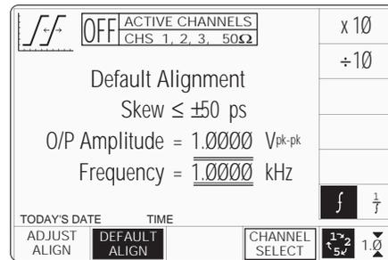
The above default screen has auto-selected 'Default Alignment', as indicated by the top line of text and the highlighted screen key on the bottom row. The unequallized (default) alignment has a maximum skew of  $\pm 50$ ps between channels. The amplitude and default frequency are also shown on the screen.
