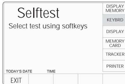
Selecting 'KEYBRD' transfers to the 'Keyboard test.' screen. This invites a user to press the front panel key to be tested, and reports on the screen the details of the last key to be pressed:
