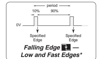
\* = For High Edge, the Duty Cycle is different, but the specified edges correspond to those shown above.
