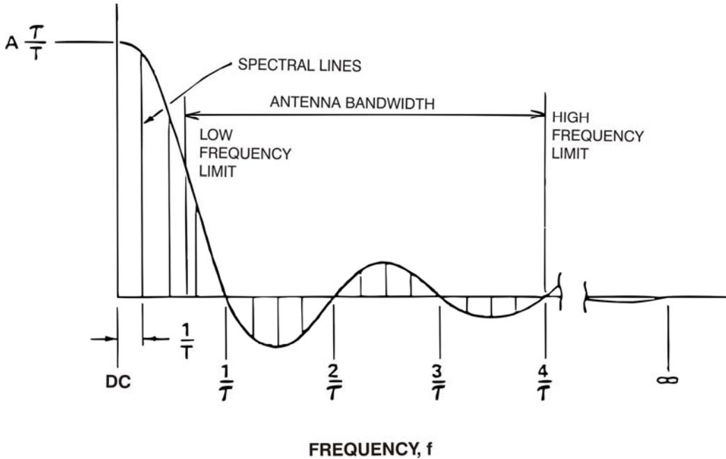
**ALTERING PULSE WIDTH / PULSE REPETITION RATE**
