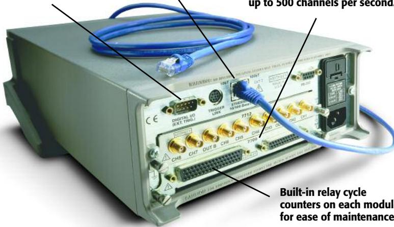
Built-in relay cycle counters on each module for ease of maintenance.
