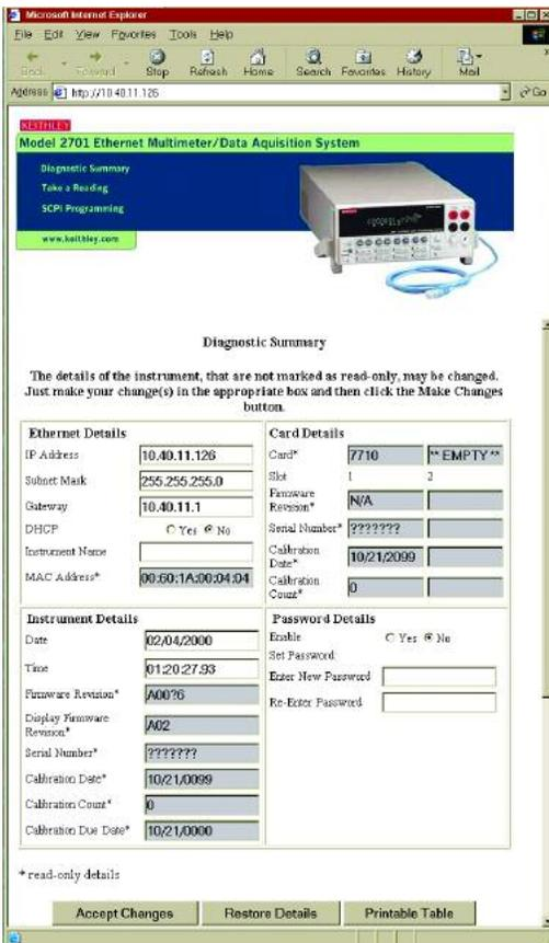
Built-in Web diagnostic tool (Model 2701 only) sends command strings and receives data over the network. It also reads and sets network parameters.
