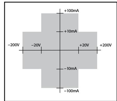
**The Model 6430 provides four-quadrant sourcing of up to 2.2W, as well as measurement sensitivity down to sub-femtoamp and microvolt levels. It can measure currents from the 1pA range (with just 0.4fA p-p noise typical) up to the 100mA range at up to 20V. Voltage ranges from 200mV to 200V are available. Current and voltage range settings define the maximum source or sink voltage or current.**
