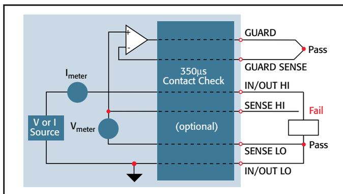
Contact check option for 4-wire or 6-wire applications
