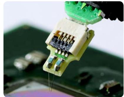
**N2887A InfiniiMax Soft touch Pro Probe Adapter** adapts from the Agilent Pro Series (36 ch) Soft touch connectorless logic analyzer foot print to the Agilent InfiniiMax I & II series probe amplifier input connectors
