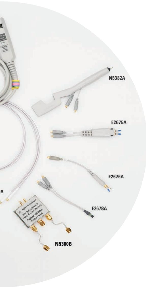
Six different InfiniiMax probe amplifiers from 1.5 GHz to 13 GHz are available for matching your probing solution to your performance and budget requirements. The 1168/69A InfiniiMax II amplifiers offer the highest bandwidth and the lowest noise floors. The 1134/32/31/30A offer a more cost efficient solution and wider dynamic range.
